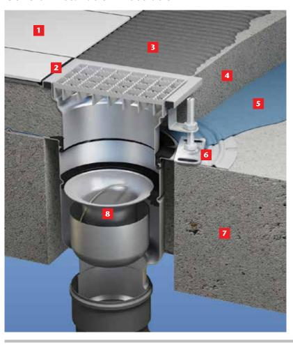
Adjustable height gully with internal FAT in suspended slab with a tile floor finish connecting into stainless pipe.
